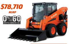
Engine gross horsepower: 64.0 hp (47.7 kW) Rated operating capacity: 1,950 lbs. (885 kg) Operating weight: 7,319 lbs. (3,320 kg)
